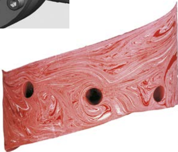
QSM compound cross section: flow division obtained by the pins of the pin-type mixing barrel
