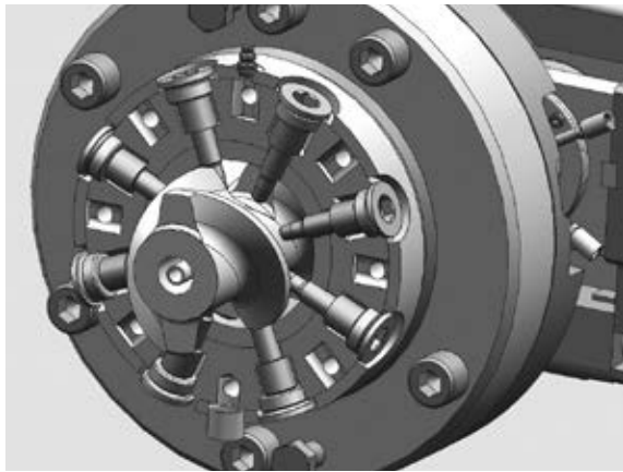
Schematic view of the cross flow mixing barrel
